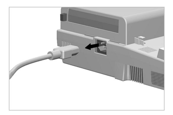
Figure 7-3. Disconnecting the Expansion Base
